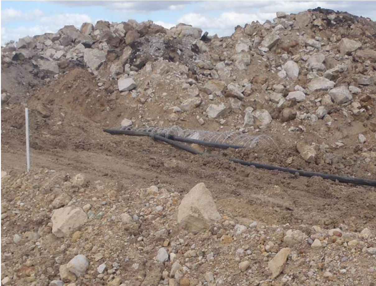
Figure 2.10 Water Curtain used to mitigate an area of spon comb in pit at WCC
